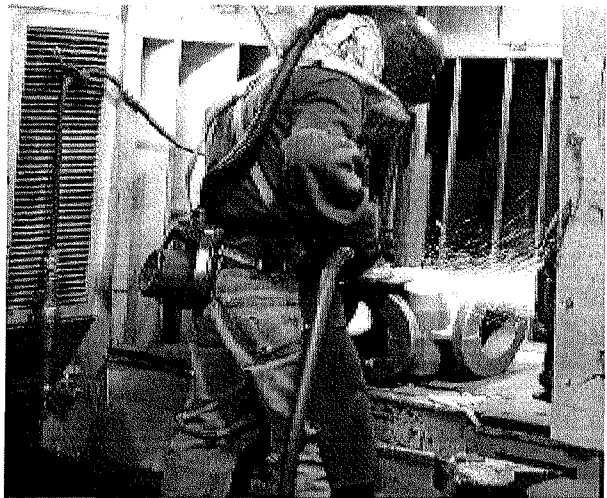
A worker grinding castings in a foundry. The work is performed in a ventilated booth to reduce the worker's exposure to silica.
